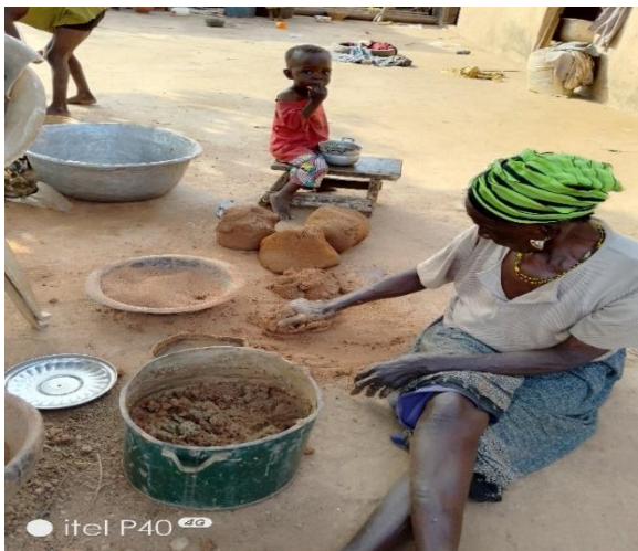
Plate 3: Kukuao community potter mixing grog with plastic clay
