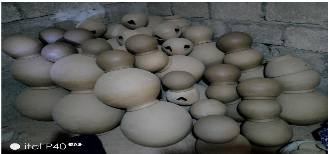
Plate 11: Pottery wares going through drying process at room temperature
