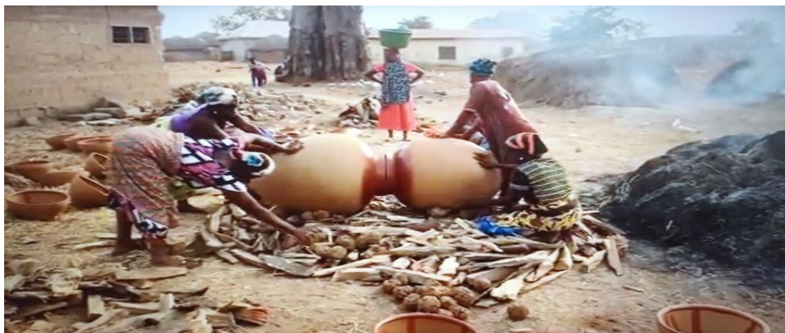
Plate 14: Positioning dry pottery wares for firing with bigger and heavier pots under and the mouths of the pots facing one another
