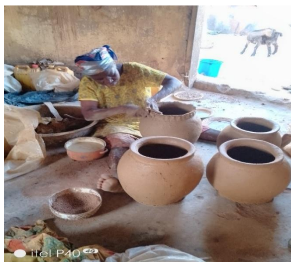
Plate 8: Coils blended to create a unified structure
