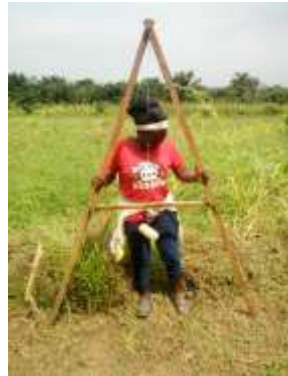
Photo 1 : contour line determination with the A-triangle Source: Blalogoé, november 2021
