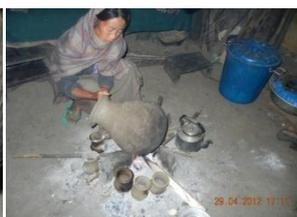
**Fig 13b:-** Warming of pots before firing
