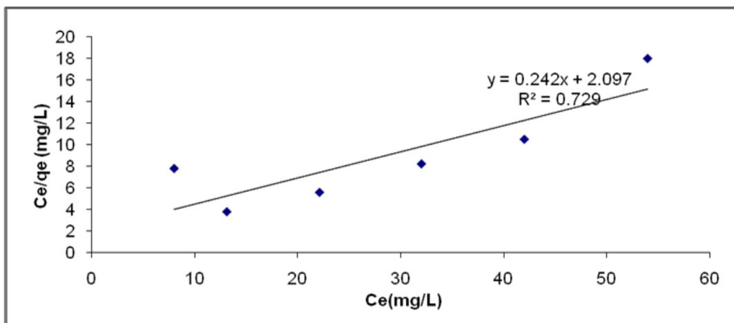
Fig 9: Langmuir Isotherm for initial concentration of Zn (II) adsorption onto UMBH
