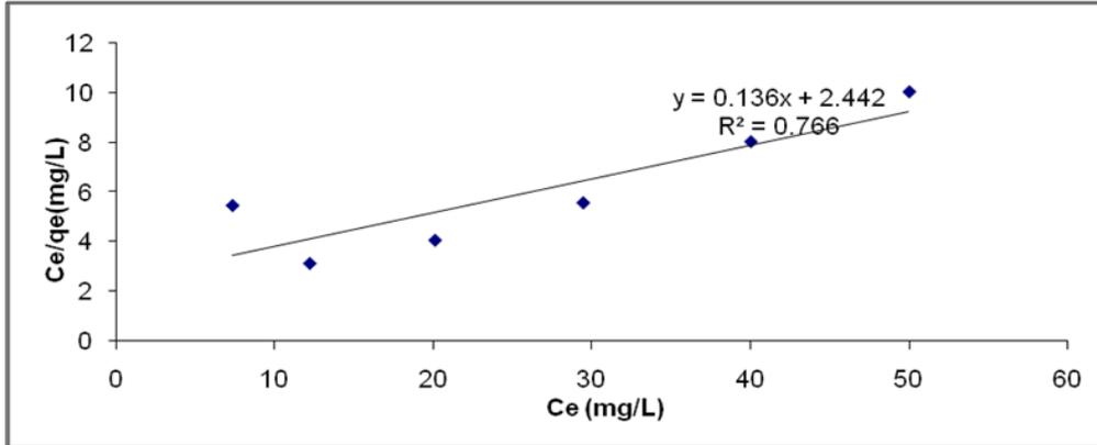
Fig 10: Langmuir Isotherm for initial concentration of Zn (II) adsorption onto EMBH
