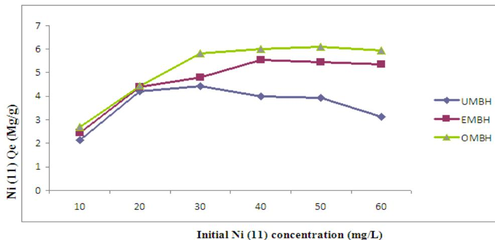
Fig 3: The effect of the initial concentration on the quantity of Ni (11) removed (Qe) onto each of UMBH, EMBH and OMBH
