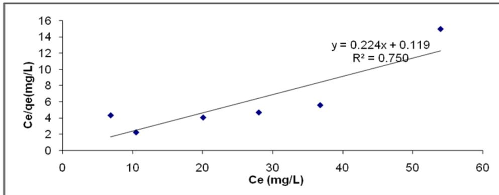
Fig 11: Langmuir Isotherm for initial concentration of Zn (II) adsorption onto OMBH
