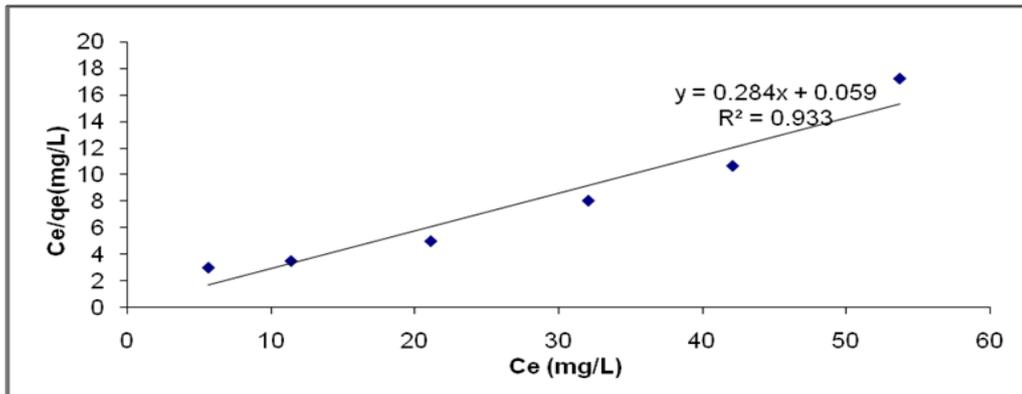
Fig 12: Langmuir Isotherm for initial concentration of Ni (II) adsorption onto UMBH
