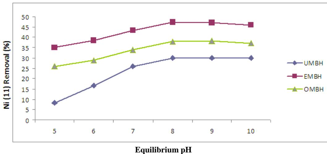
Fig 6: Effect of solution pH on the removal of Ni (II) onto each of UMBH, EMBH and OMBH
