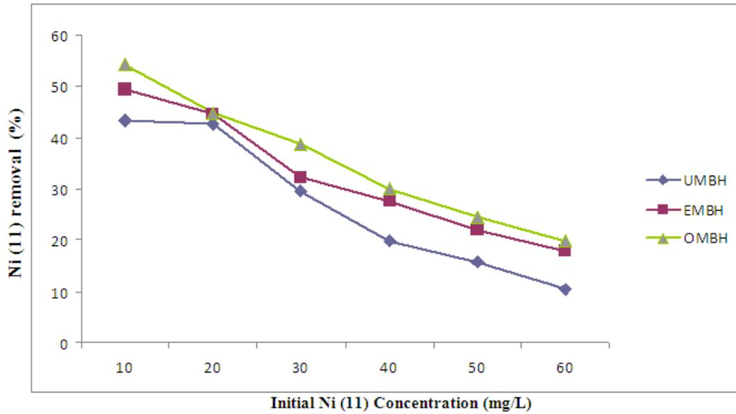
Fig 4: Effect of initial Concentration on percentage removal of Ni (II) onto each of UMBH, EMBH and OMBH
