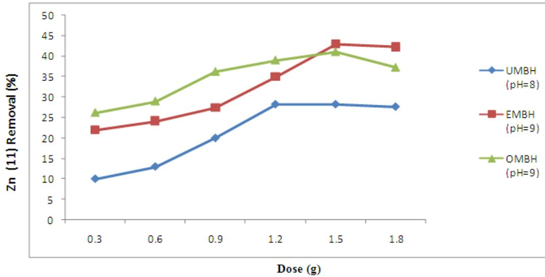
Fig 7: Effect of adsorbent dose on the removal of Zn (II) onto each of UMBH, EMBH and OMBH
