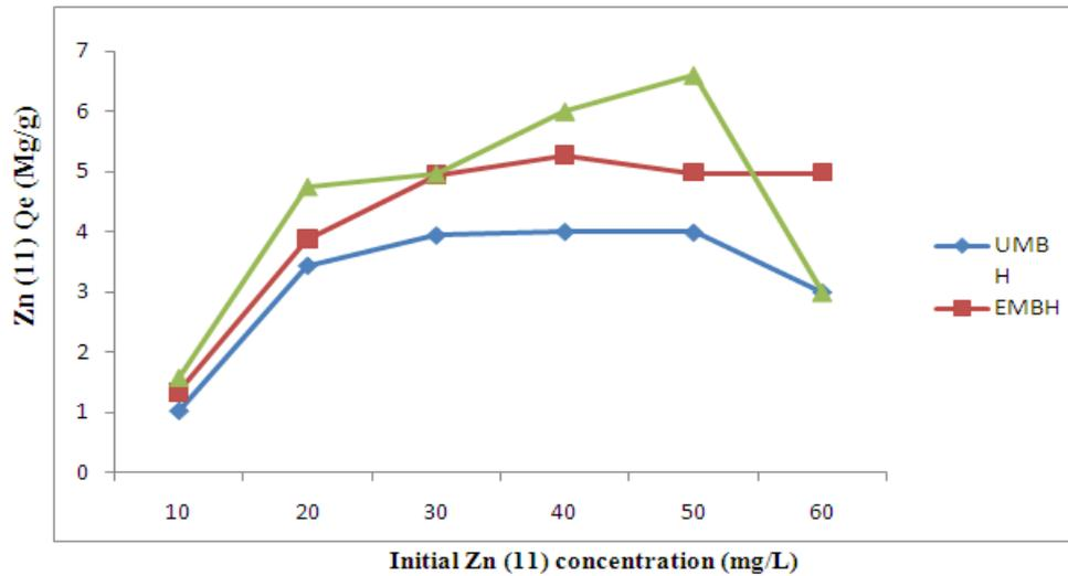
Fig 1: The effect of initial concentration on the quantity of Zn (11) removed (Qe) onto each of UMBH, EMBH and OMBH
