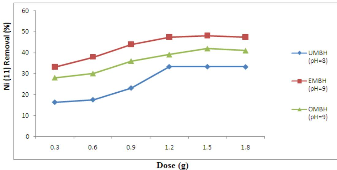
Fig 8: Effect of adsorbent dose on the removal of Ni (II) onto each of UMBH, EMBH and OMBH
