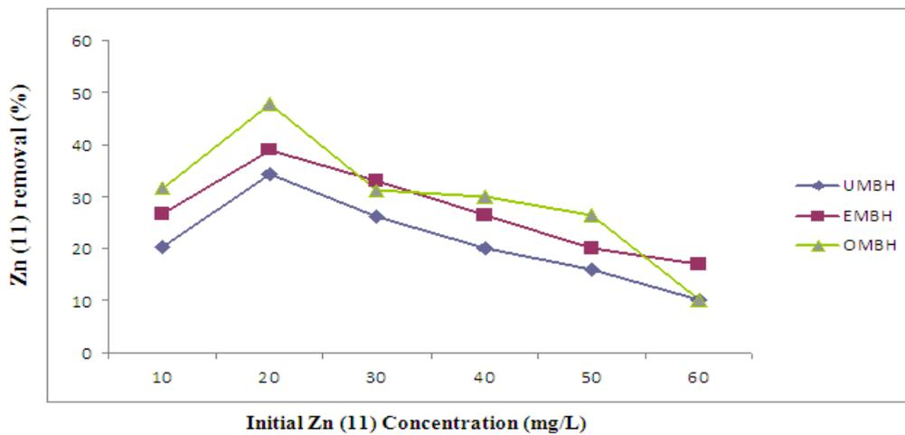
Fig 2: Effect of Initial Concentration on the removal percentage of Zn (11) onto each of UMBH, EMBH and OMBH
