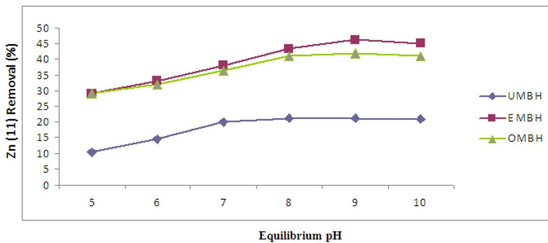
Fig 5: Effect of solution pH on the removal of Zn (II) onto each of UMBH, EMBH and OMBH
