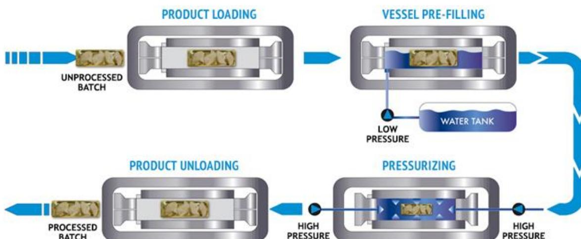
**Figure 1: Diagram of operation of HPP unit.**
