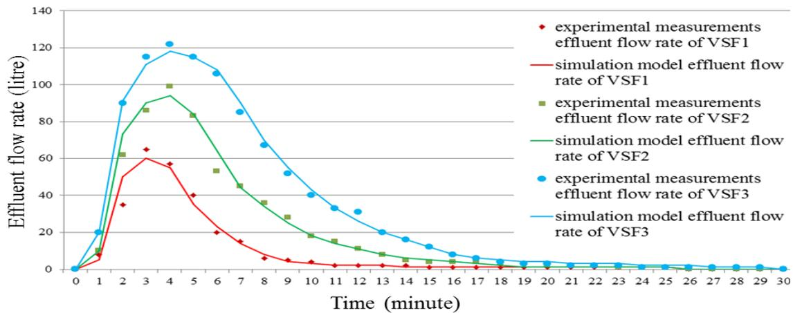
Figure 3 Hydrograph of experimental measurement and simulation model of effluent flow rates of VSF CW 1, 2 and 3.
