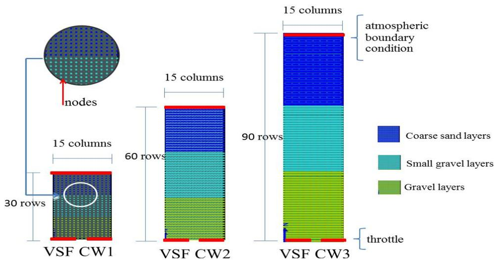
Figure 2 The 2D finite element mesh of VSF CW1, 2 and 3 were generated by HYDRUS-2D.
