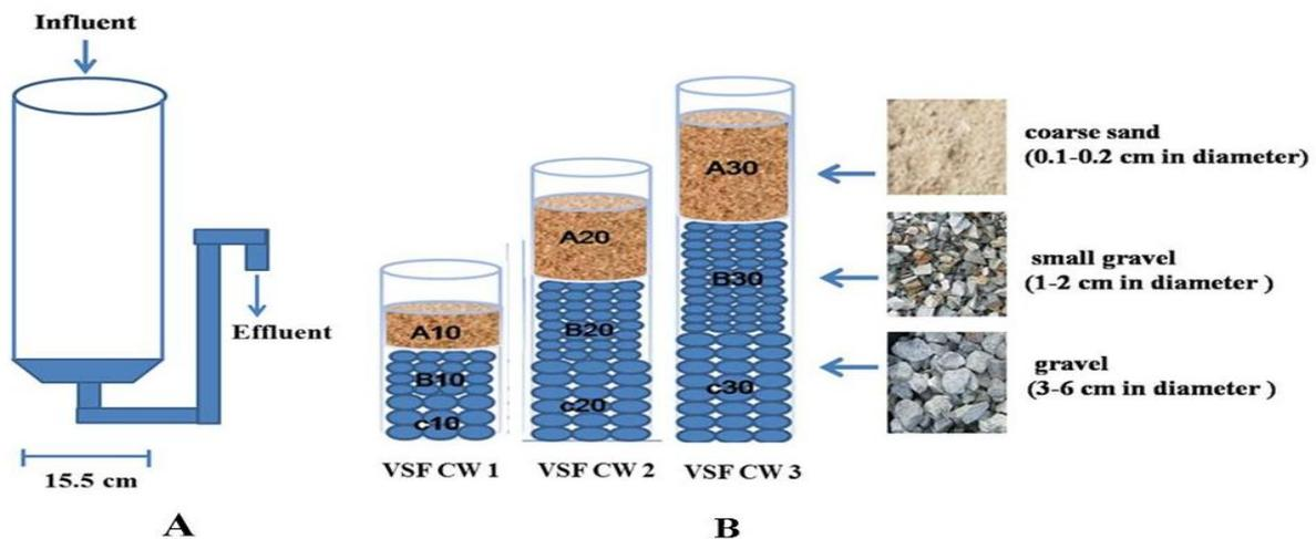
Figure 1(A) VSF CW was constructed from poly vinyl chloride pipes. (B) Inside VSF CW contained 3 types of media. A: coarse sand (0.1-0.2 cm in diameter), B: small gravel (1-2 cm in diameter), C: gravel (3-6 cm in diameter), and number 10, 20 and 30 are media depths (cm).
