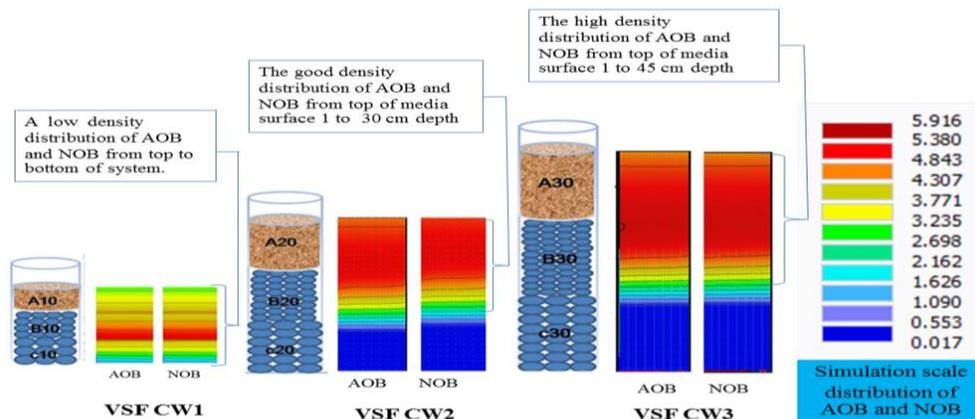
Figure 6 Simulation scale of distribution of ammonia-oxidizing bacteria (AOB) and nitrite-oxidizing bacteria (NOB) in the VSF CW1, 2 and 3 at day 30.
