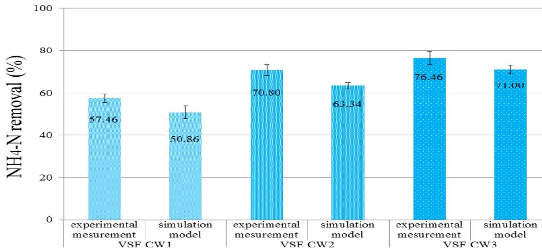
Figure 5 Experimental measurements and the model simulations of average ammonia nitrogen removal efficiencies by VSF CW 1, 2, and 3.
