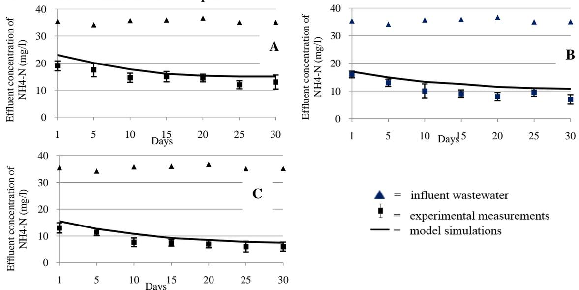
Figure 4 Effluent concentrations of ammonia nitrogen removal by VSF CW1 (A), VSF CW 2 (B) and VSF CW3 (C).
