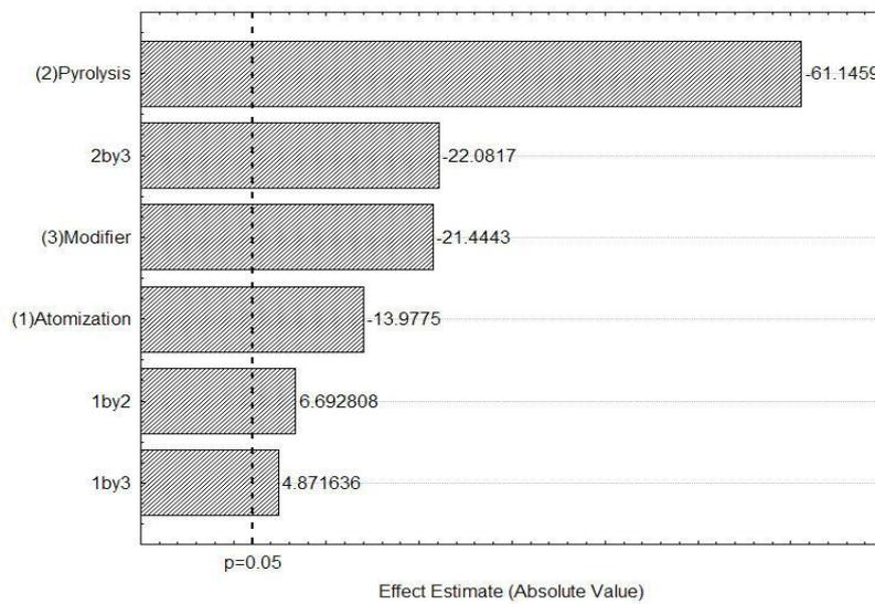
Fig. 3. Pareto chart obtained in factorial design for Cr in serum samples.
