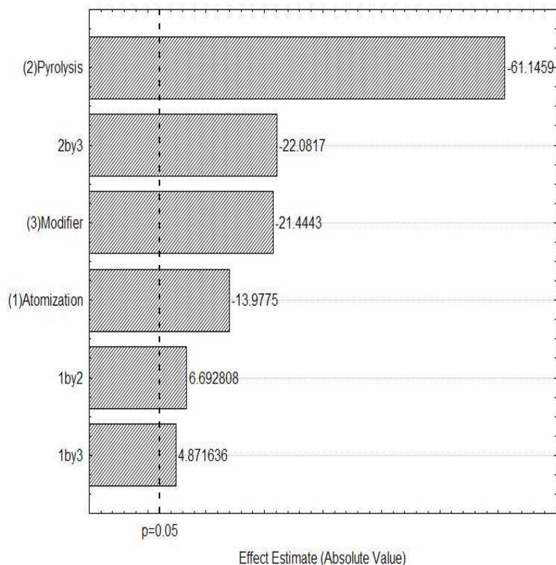
**Fig. 1.** Pareto chart results for the factorial design for Sb determination.
