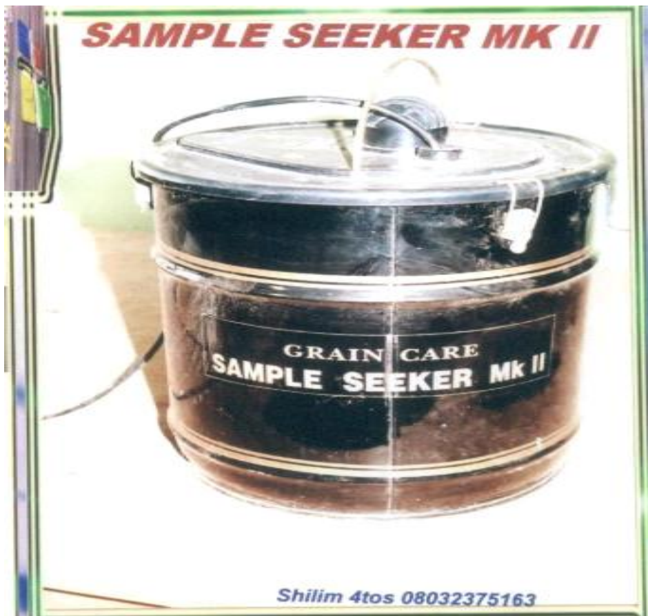
Plate 2. Sample of a grain seeker used for collection of paddy grains samples.
