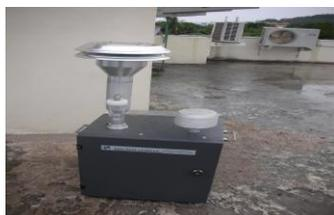
**Fig -2: Fine dust sampler**
