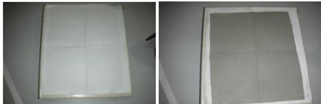
**Fig 3 : Filter papers before and after sampling**
