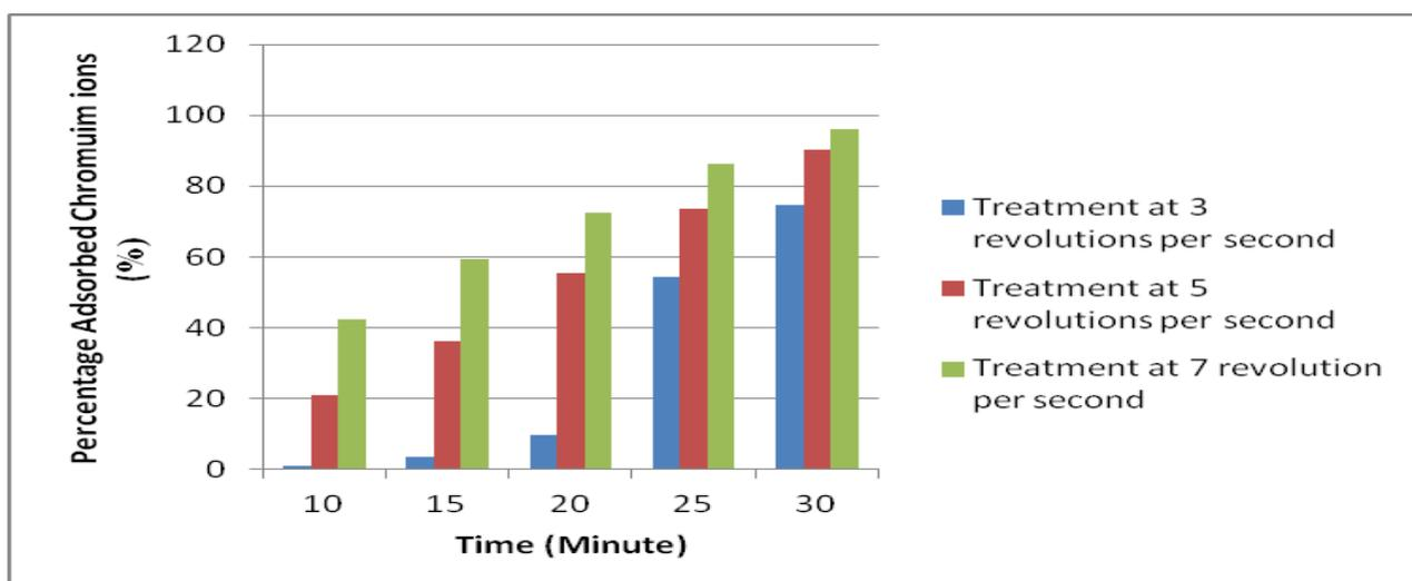
**Figure 2:** Chart displaying Effects of Treatment time on Chromium ion removal using Moringa Oleifera Pods at different stirring speed.
