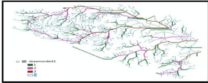
Figure 1.6: Stream Network with Threshold value  $> 100$  overlay with Labisriver.shp data
