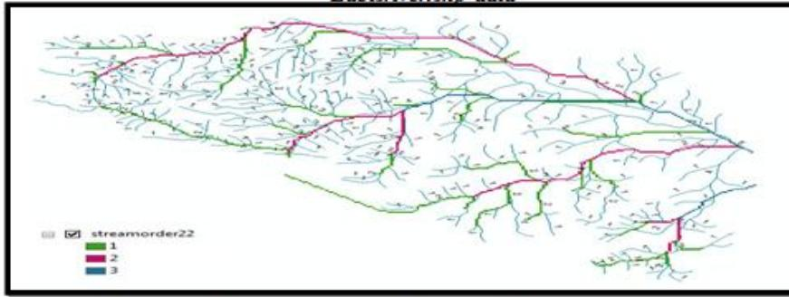
Figure 1.7: Stream Network with Threshold Value  $> 200$  overlay with Labisriver.shp data
