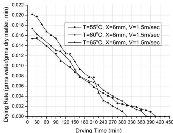
**Fig. 6: Variation of Drying Rate with drying Time at different temperatures and velocity (1.5m/s) for slice thickness 6mm.**
