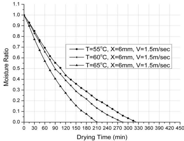
**Fig. 5: Variation of Moisture Ratio with drying Time at different temperatures and velocity (1.5m/s) for slice thickness 6mm.**
