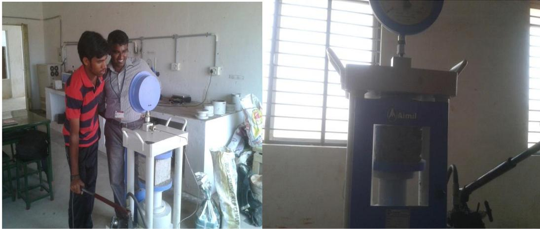
**Fig 2.0 Compression test of M20 concrete cube**
