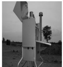
Figure 2.1: High Volume sampler installed at the proposed site
