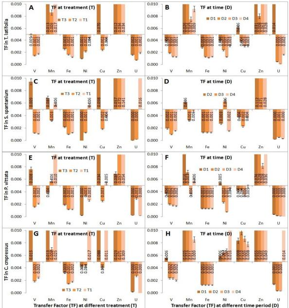
Figure – 11: A-H: Transfer Factor capabilities of selected plants during the Phyto-remediation of Uranium mine tailing at EPTRI, Hyderabad (A.P.). All the values are mean of three treatment and bars represents •  $\pm$  SE (n = 5). D1 - 1<sup>st</sup> – month data; D2 - 2<sup>nd</sup> – month data; D3 - 3<sup>rd</sup> – month data; D4 - 4<sup>th</sup> – month data; dw – dry weight; T1 – Treatment 1; T2 – Treatment 2; T3 – Treatment 3.
