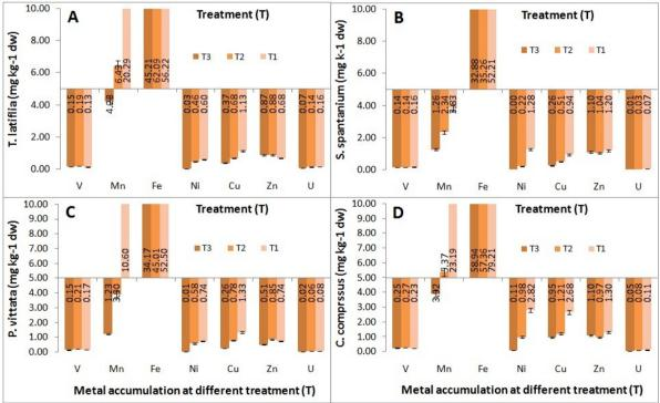
Figure – 10: A-D: Metal bio-concentration (mg kg<sup>-1</sup> dw) of selected plants during the Phyto-remediation of Uranium mine tailing at EPTRI, Hyderabad (A.P.). All the values are mean of replicate samples and bars represents •  $\pm$  SE (n = 5). (T3 – Treatment 3; T2 – Treatment 2; T1 – Treatment 1; dw – dry weight).
