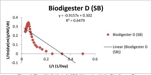
Figure 6: Plot of 1/t(ln(dyt(ml/gVM)/dt)) against 1/t for Bio-digester D
