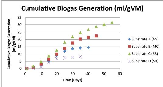
Figure 2: Cumulative Biogas Generation (ml/g VM) with Time of the various Substrates
