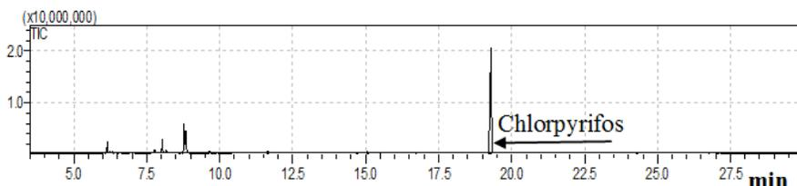
Fig.5 GC-MS chromatogram of Chlorpyrifos without Ag nanoparticle
