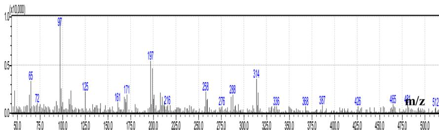
Fig.4 Mass spectrum of Chlorpyrifos has been shown.
