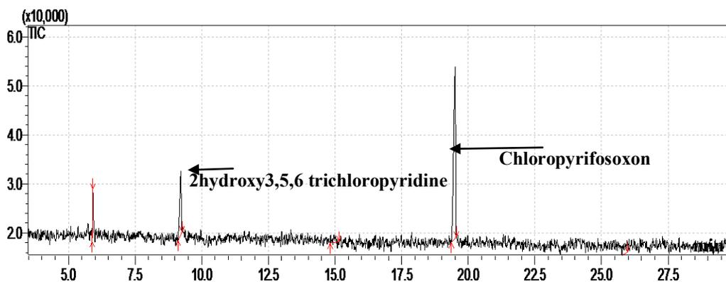
Fig.1 GC-MS chromatogram of ozonated Chlorpyrifos
