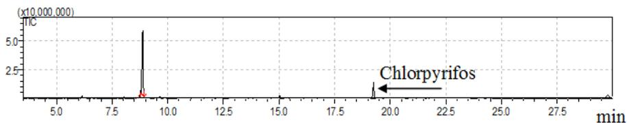
Fig.7 GC-MS chromatogram of Chlorpyrifos with Ag nanoparticle
