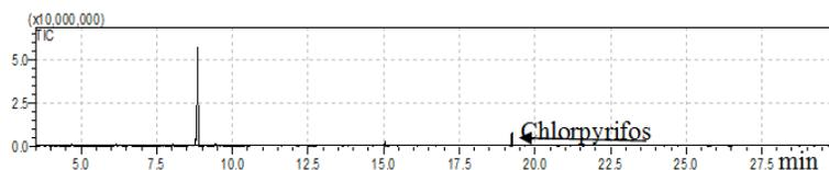
Fig.8 GC-MS chromatogram of Chlorpyrifos with Ag nanoparticle.
