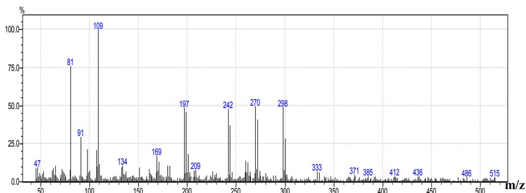
Fig.2 Mass spectrum of Chlorpyrifos oxon. Molwt.333
