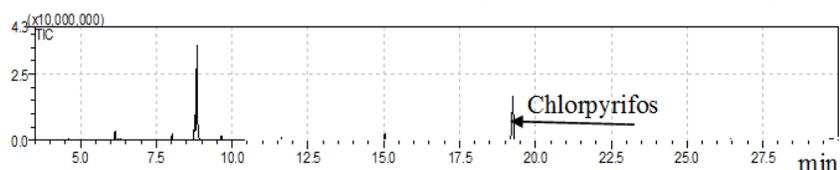
Fig.6 GC-MS chromatogram of Chlorpyrifos with Ag nanoparticle
