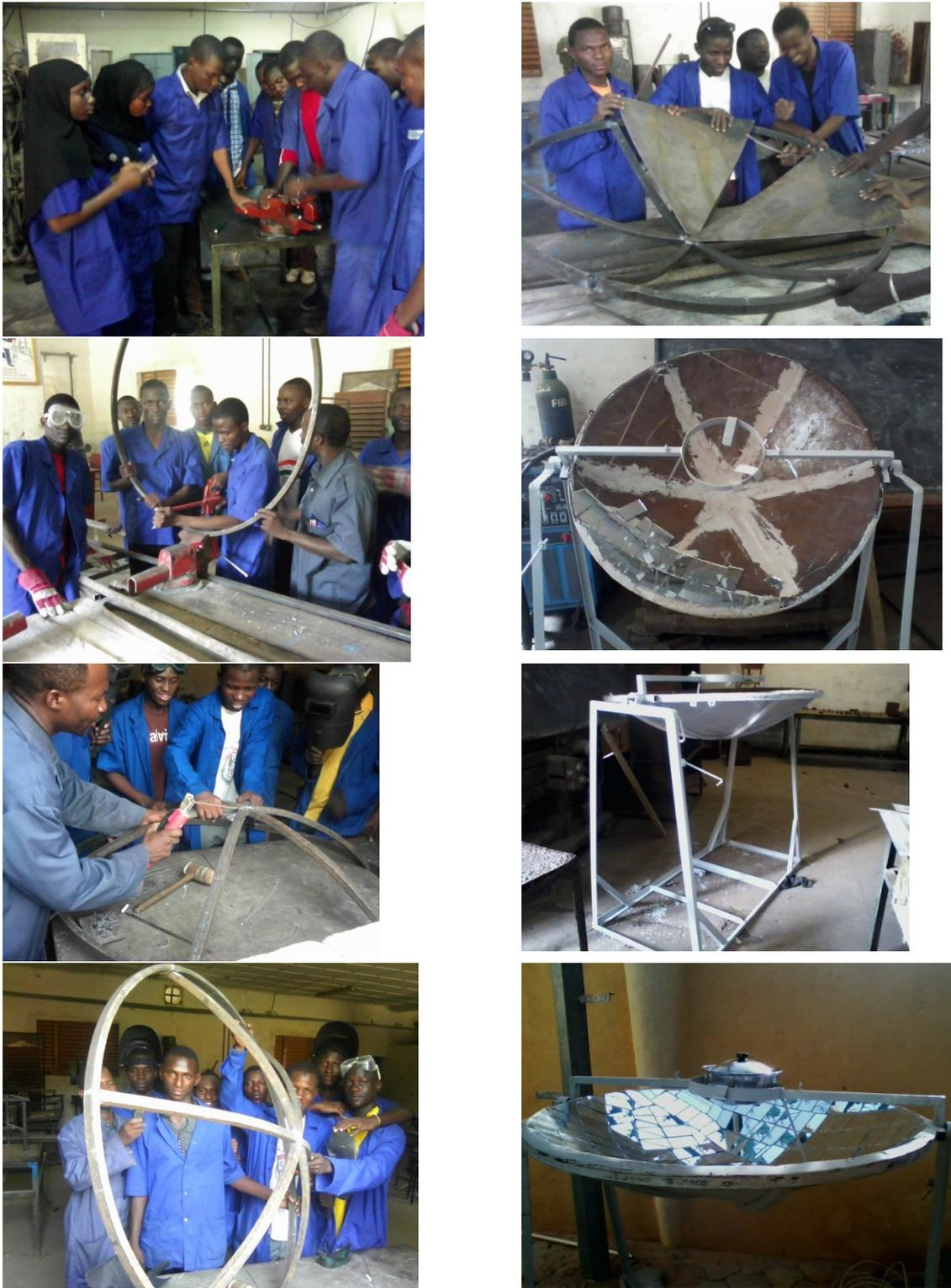
Fig. 1.6 Students in practical metallic construction (Solar cooker)
