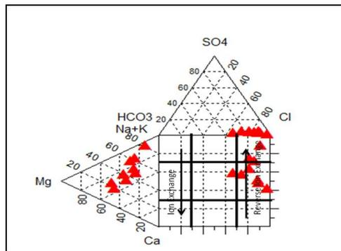
Fig.4.4. Durov Plot Showing Ion Exchange Process
