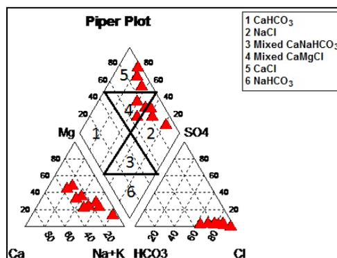
Fig.4.5. Piper Plot Showing Hydrochemical Facies
