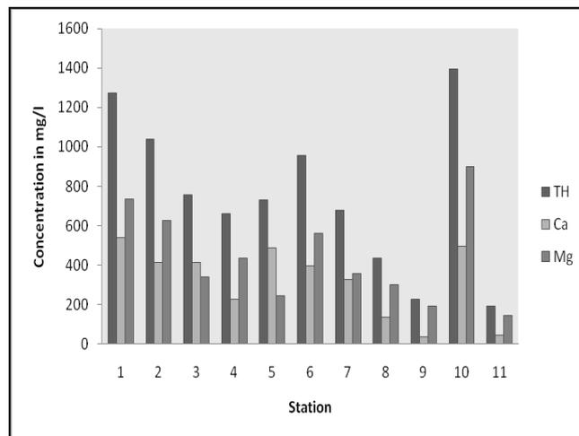
Fig.4.2 Concentration of Total hardness
