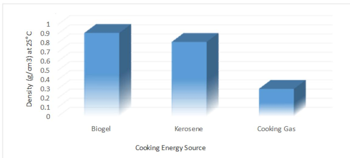
Figure 3c: Graphical representation of each cooking energy source density (g/cm<sup>3</sup>) at 25 °C
