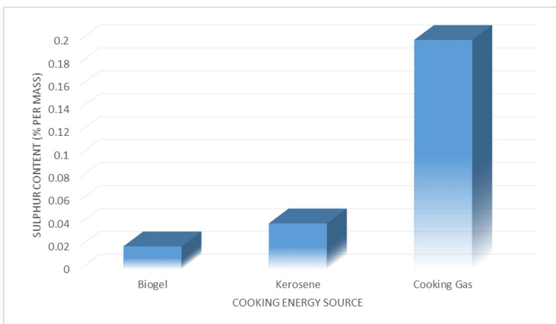
**Figure 3d:** Graphical representation of each cooking energy source density sulphur content (% per mass)
