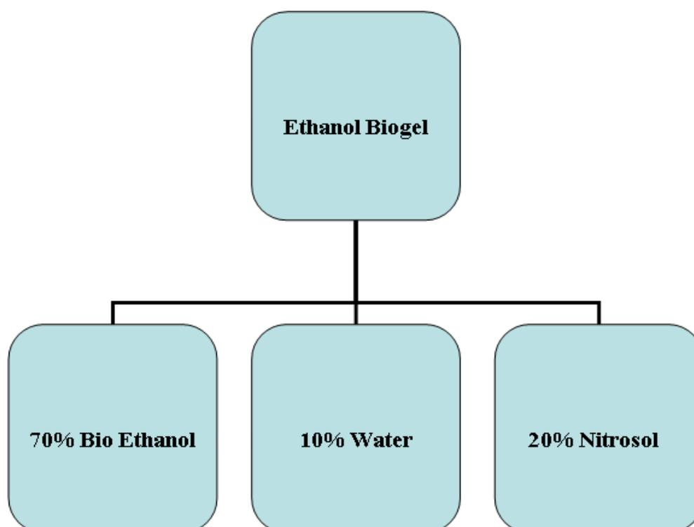
**Figure 2:** A flow diagram representing materials and formulation for production of ethanol biogel; an alternative source for cooking. Three ingredients as shown above were used for the production of the ethanol biogel. These are very much in abundance and thus describing the cheap production status and consistency of the product.
