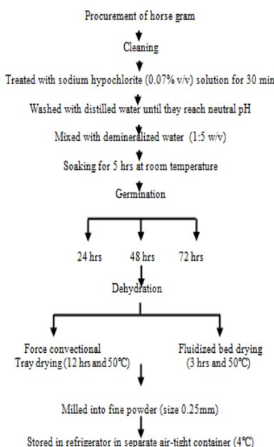
**Figure 1.** Flowchart showing the process for germination and dehydration of horse gram seeds
