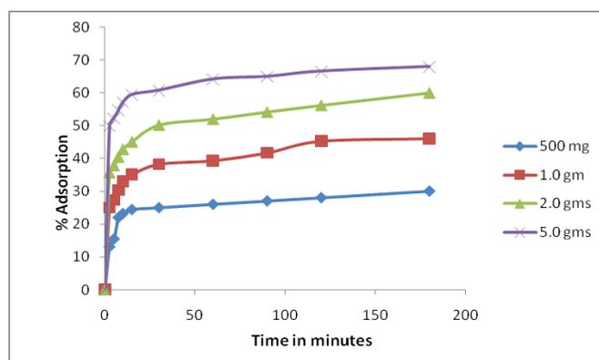
**Fig. -1 Effect of time on % adsorption by S-IV Fig-2 Plot of adsorption capacity vs. time for Pb<sup>2+</sup>**
