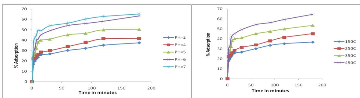
Fig-3 Effect of pH on % adsorption of Pb<sup>2+</sup> Fig-4 Effect of temperature on % adsorption of Pb<sup>2+</sup>
