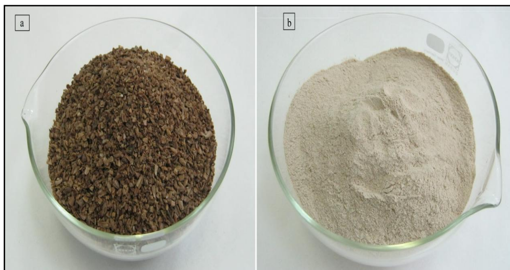
Fig 1: olive cake in form of granular (a), and olive cake in form of olive cake powder (b).
