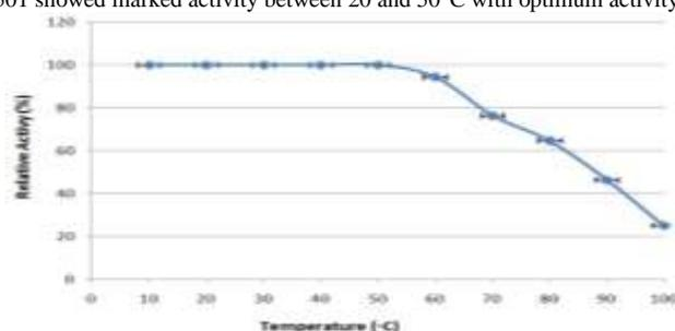
Figure 5: Effect of temperature on cholesterol oxidase activity
