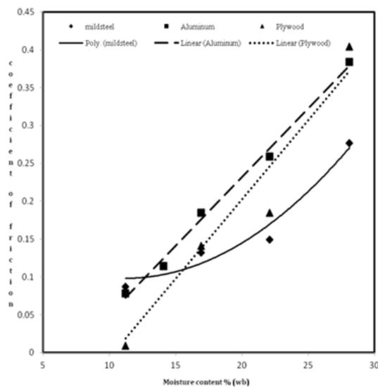
Fig. 1:Friction coefficients of BGG at different moisture contents
