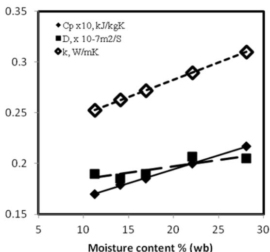
Fig.3: Variation of thermal properties of BBG with moisture
