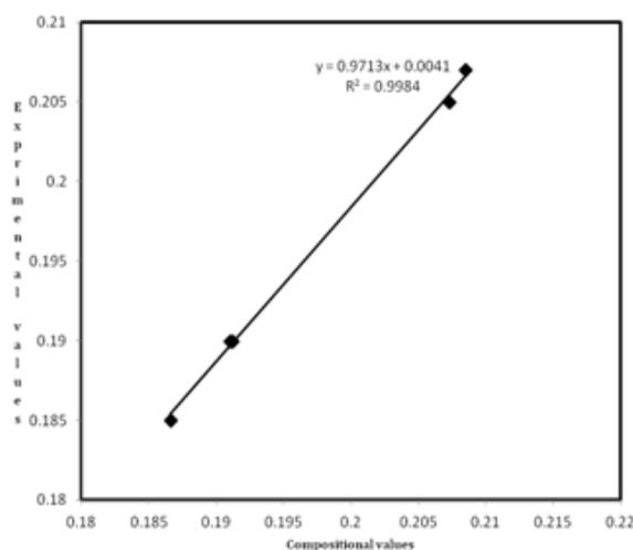
Fig.5: Correlation between experimental and compositional values for thermal diffusivity(x10<sup>-7</sup> m<sup>2</sup>/s)
