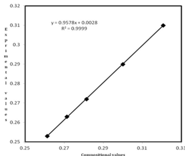
**Fig. 6:** Correlation between experimental and compositional values for thermal conductivity(W/mK)
