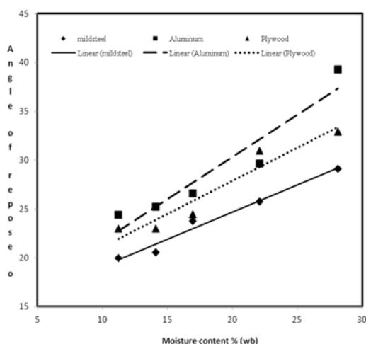
Fig. 2:Angle of repose of BGG at different on various surfaces moisture contents on various surfaces
