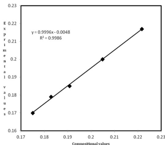
Fig. 4: Correlation between experimental and content compositional values for specific heat ( $\times 10 \text{ kJ/kgK}$ )
