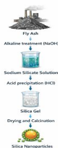
Figure – 1 AI-assisted flow diagram of fly ash-derived silica nanoparticle extraction using chemical digestion and precipitation techniques, created and modified by the authors.
