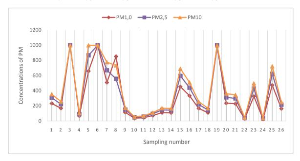
Figure 9: Concentrations of PM1, PM2, 5 and PM 10 at the melt reactor
