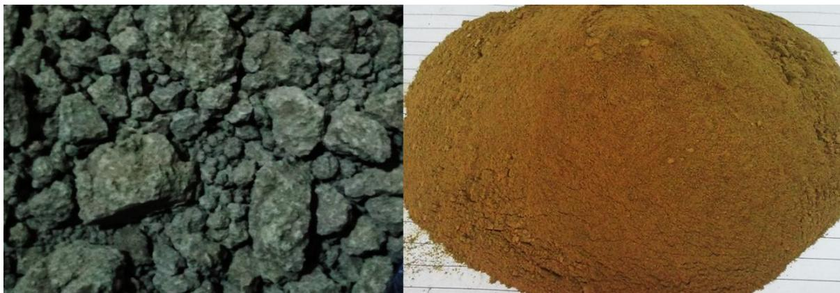
Figure 2: Crushing, grinding and sieving green clay
