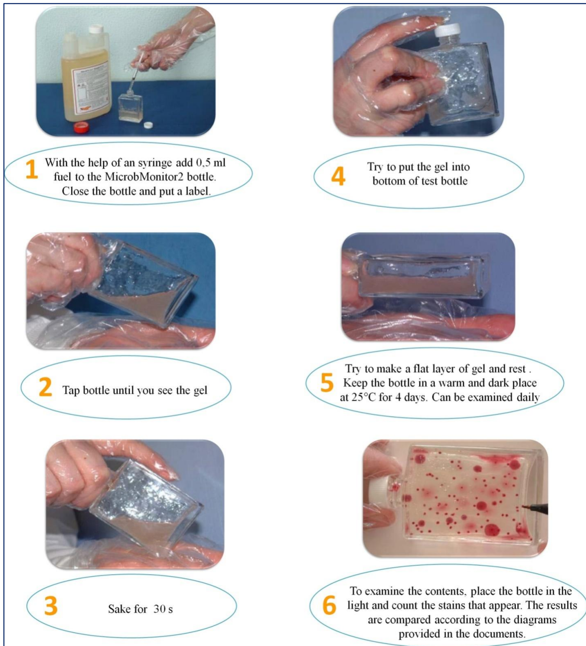
Fig.3 - Aircraft fuel test procedure with MICROBMONITOR2 [10]
