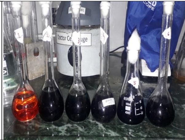
Fig.6. Estimation of alcohol by Dichromate method
