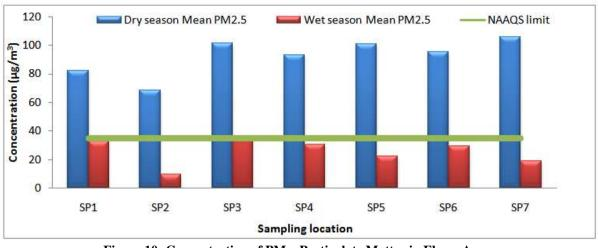
Figure 10: Concentration of PM<sub>2.5</sub> Particulate Matter in Eleme Area
