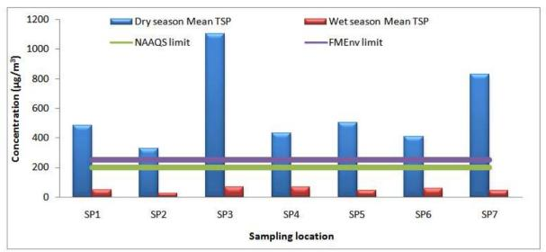
Figure 8: Concentration of Total Suspended Particulate Matter in Eleme Area
