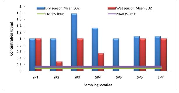
Figure 1: Concentrations of Sulphur Dioxide in Eleme Area
