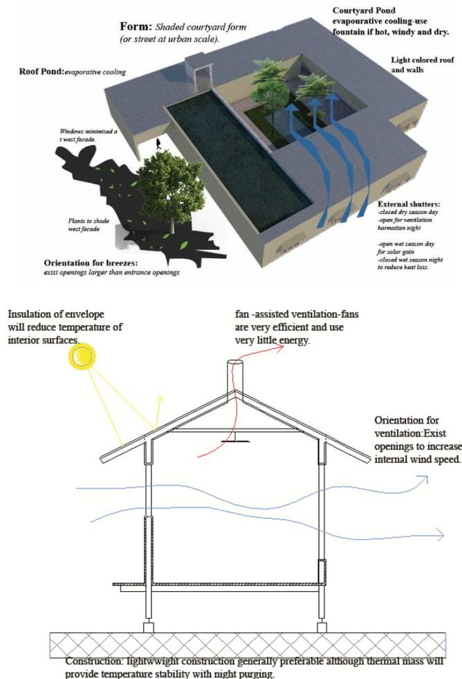
**Figure 3.1.** Showing energy efficient strategies for hot-dry and hot-humid climate ‘rule of thumb 82-85’
