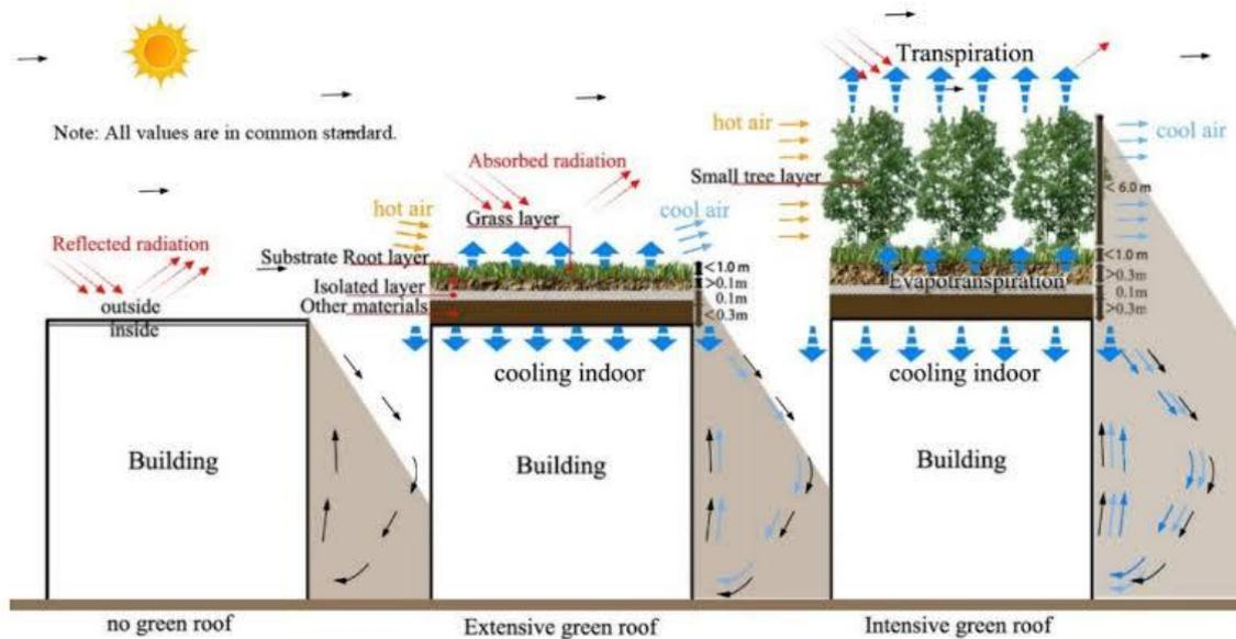
**Figure 4.1a** a schematic structure of an extensive green roof and intensive green roof, and the cooling mechanism in the daytime.(Zhang, He, Zhu, & Dewancker, 2019)
