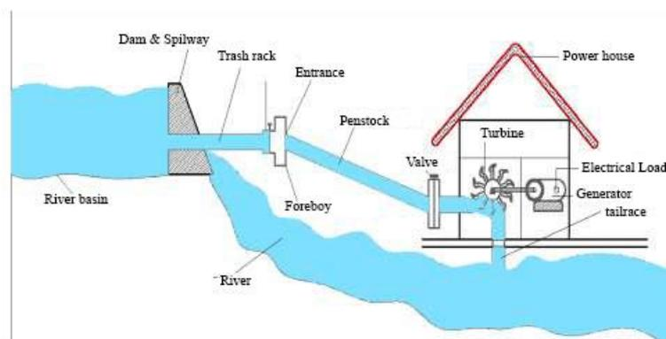
Figure 4.5. Showing a schematic diagram of a Micro-Hydro power house. (Hoxha et-all, 2017)
