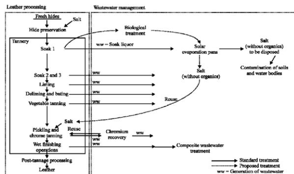
**Fig 1.2 Simplified leather production chain and management of the effluent associated.**
