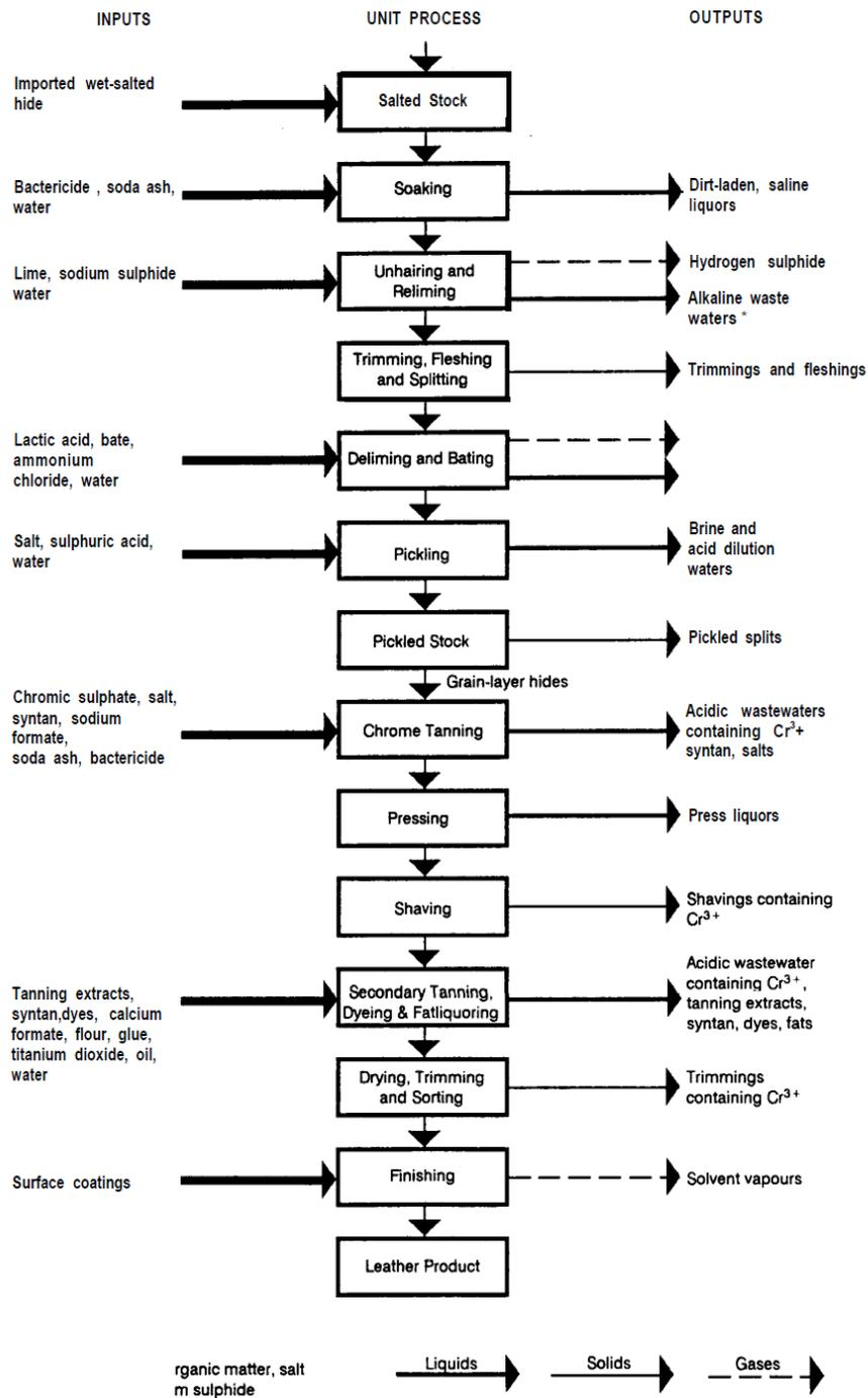
Fig 2.1 Flow diagram of leather making process.
