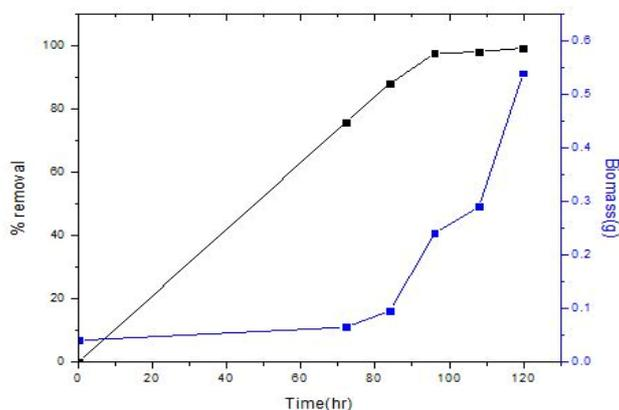
**Fig 4.3 Effect of biomass on removal of Chromium (VI) at 100ppm with respect of time.**
