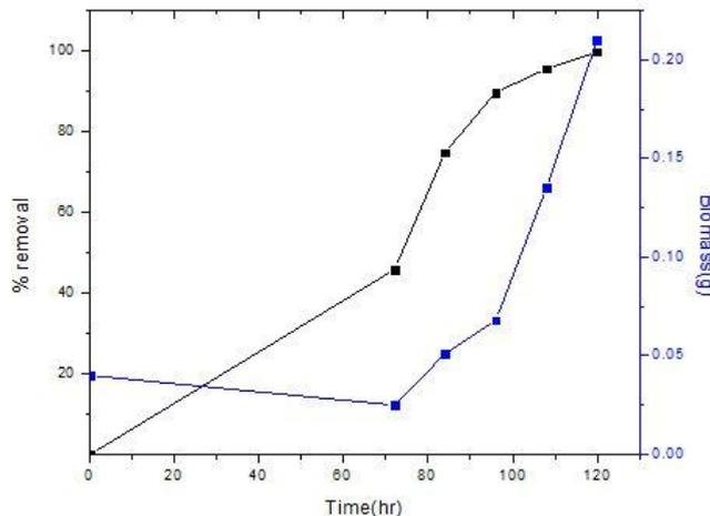
**Fig 4.7 Effect of biomass on removal of Cr<sup>6+</sup> (500ppm) with respect of time**
