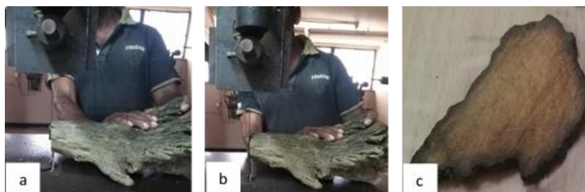
Figure no 2: Sample preparation for the taking of optical microscopic images (a, b; Preparation of sunken timber samples using power saw, c; Prepared sunken timber sample for microscopic images).
