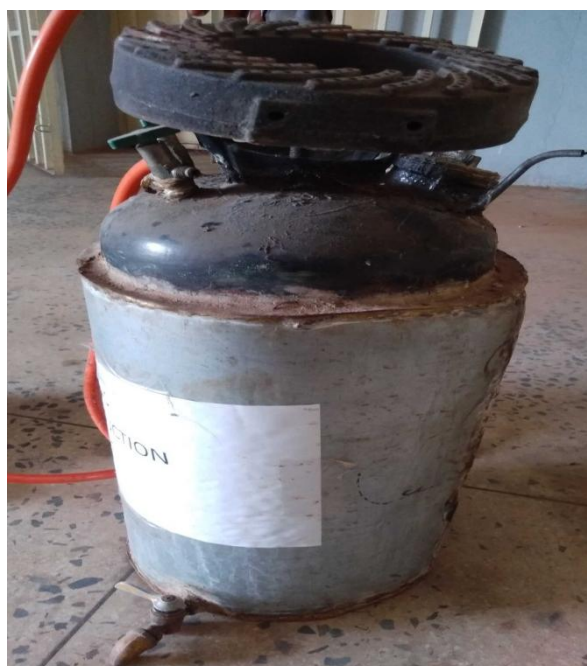
Figure A1: designed and constructed digester
