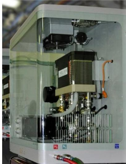
**Figure10.** Polymer Electrolyte fuel cell generating power of 1 kW and 1kW heat
