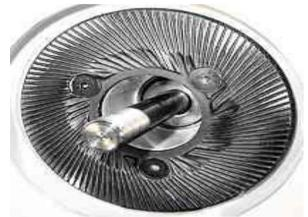
Figure 1: The Rotating Burr or plate
