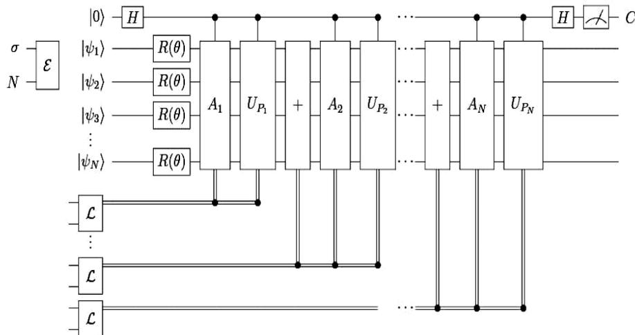
The First part of the circuit above is the epsilon function call, which derives the Eigen vectors of the quantum operator based on volatility and the number of periods. Here epsilon requires four elementary calculations and solving for Eigen vectors of a matrix.
