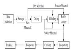
Figure 5.1 Flow diagram of biomass briquette production
