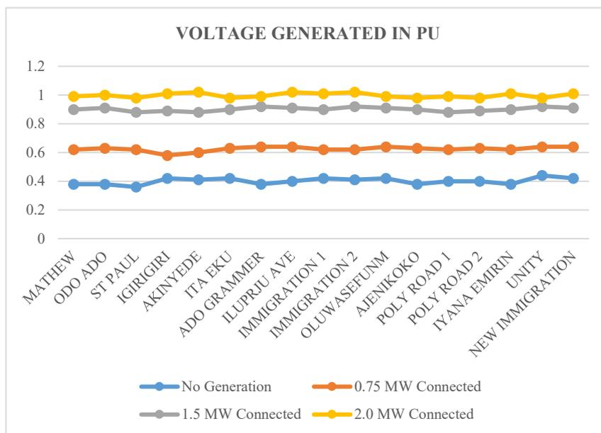
Fig. 4: Steady State Voltage Result of Primary feeder with/without DG with GA
