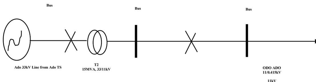
Figure 2: Schematic Representation of the Primary 11/0.415kV Injection Substation
