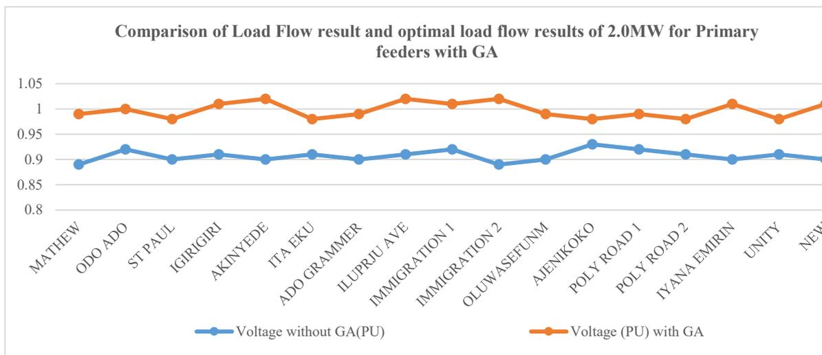
**Fig. 5. Comparison of optimal load flow results when 2.0 MW was integrated into primary distribution network feeders with and without GA**
