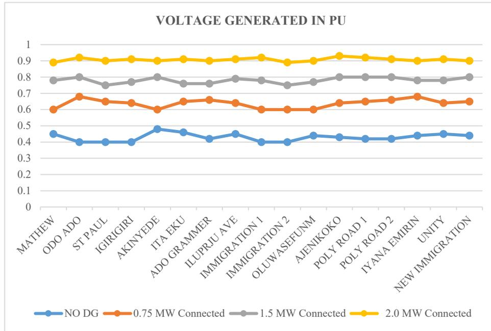
Fig. 3. Steady State Voltage Result of Primary feeder with/without DG without GA
