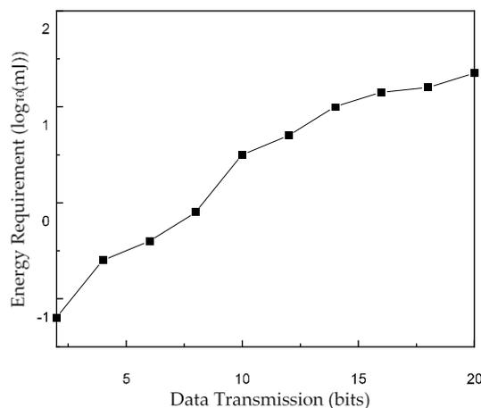
**Fig. 8. Energy requirement of sensor node during data transmission with increasing number of bits.**
