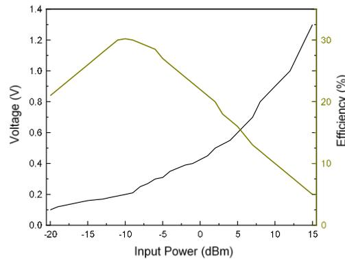
Fig. 4. Variation of input power including relative effect of efficiency and voltage.
