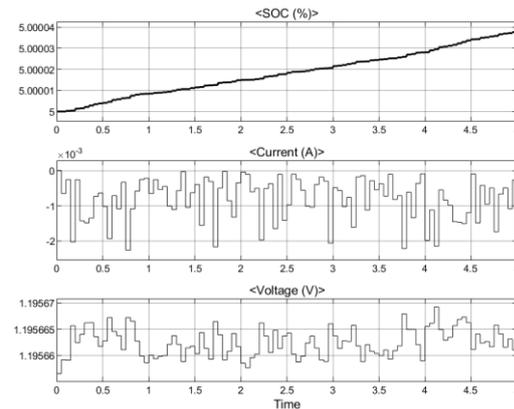
Fig. 6. The voltage, current, and the state of charge response of the battery with the variation of time.
