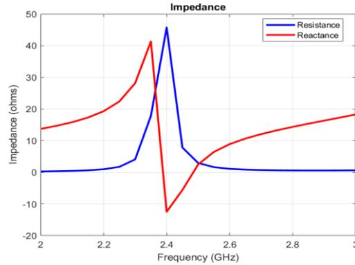
Fig. 3. Impedance of the antenna in RF-EH circuit.
