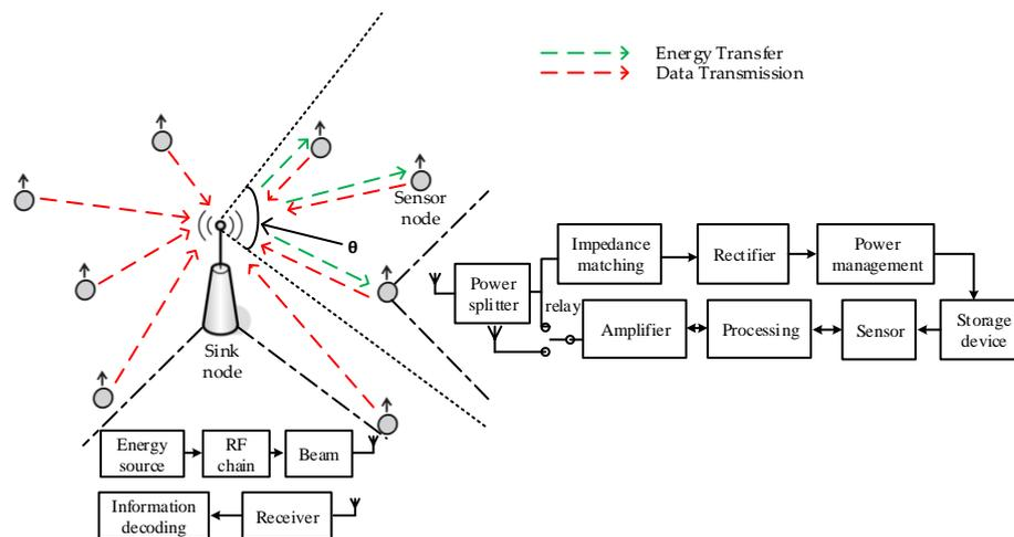
Fig. 1. Network model describing data transmission and energy transfer at a certain beamforming angle.
