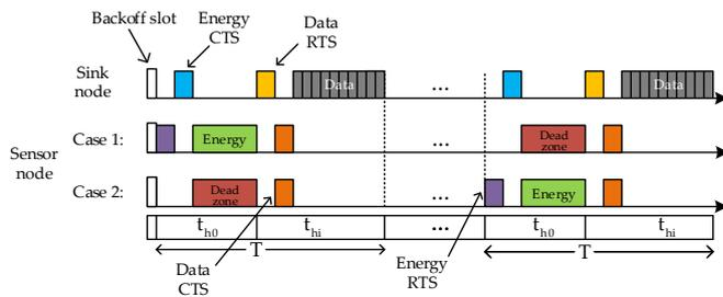
Fig. 2. Proposed TDMA protocol introducing the dead zone.
