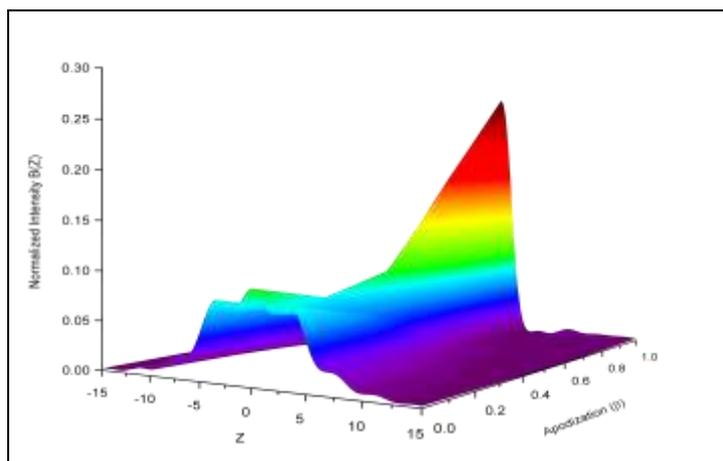
Fig. 5 3D Intensity distribution for two zone aperture at a =0.7 under highest degree of defocus and primary spherical aberration
