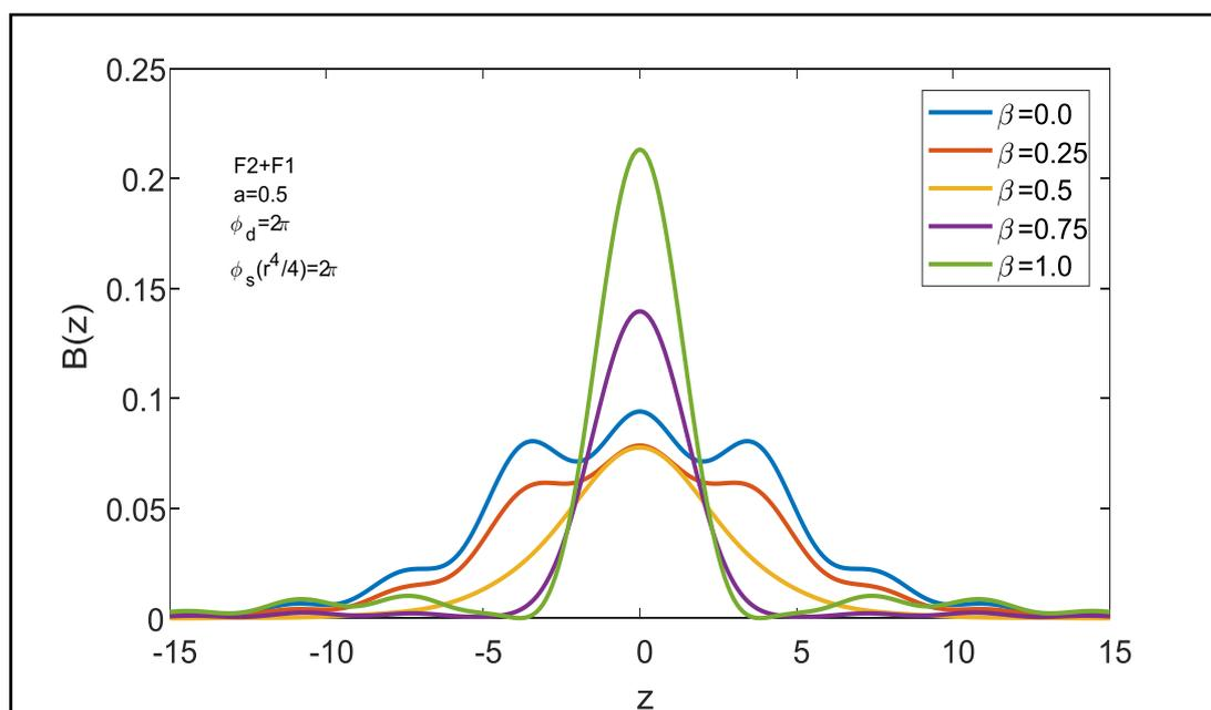
Fig. 3 Intensity distribution curves for two zone aperture with  $a=0.5$
