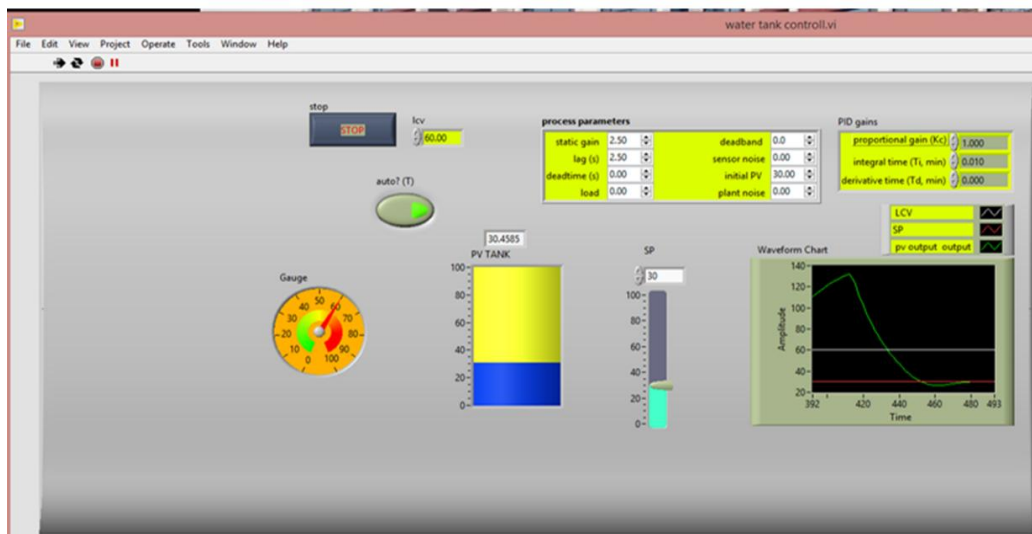
Figure no 7: Advance LABVIEW diagram for Water Level Condition
