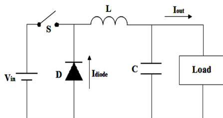
Fig.1. Buck converter
