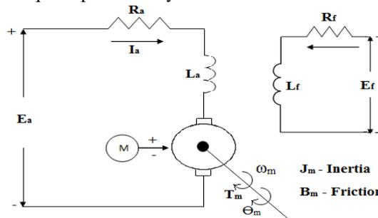
Fig.4. Equivalent circuit of separately excited DC motor
