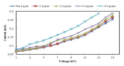
Fig. 11: Leakage current as a function of applied voltages when different layers of insulation paper are held between the electrodes in oil with 100ppm DBPC concentration.
