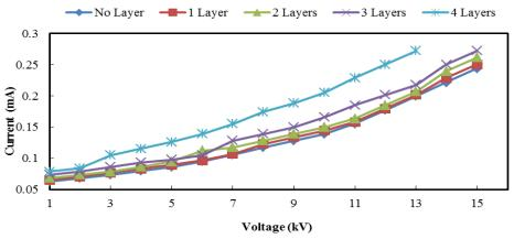
Fig. 6: Leakage current as a function of applied voltages when different layers of insulation papers are held between the electrodes in oil with 25 ppm DBDS concentration.
