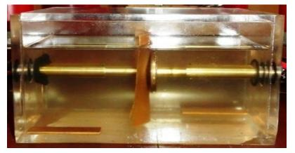
Fig. 4: Cell with insulation paper held between the plane-plane electrodes.
