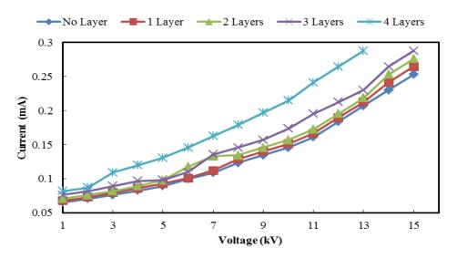
Fig. 10: Leakage current as a function of applied voltages when different layers of insulation paper are held between the electrodes in oil with 50ppm DBPC Concentration.
