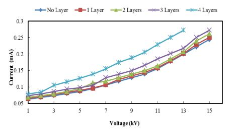
Fig. 7: Leakage current as a function of applied voltages when different layers of insulation paper are held between the electrodes in oil with 50ppm DBDS concentration.
