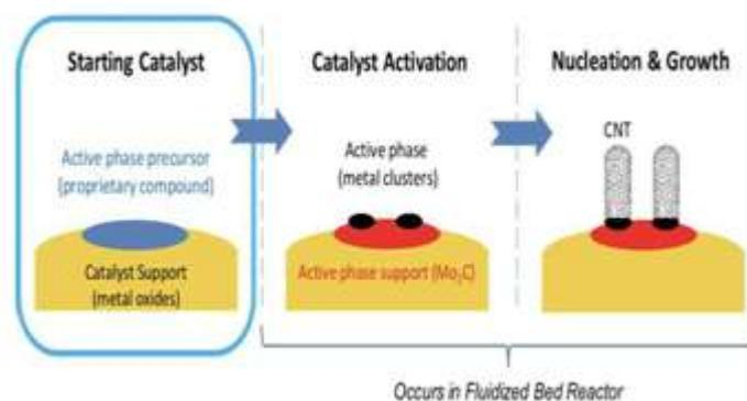
Figure 1 Chemical vapor deposition
