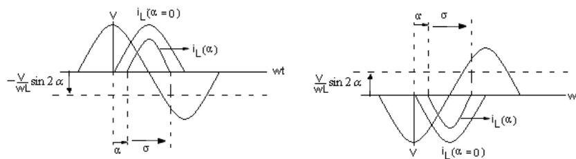
Fig. 2. Firing Delay Angle Control
