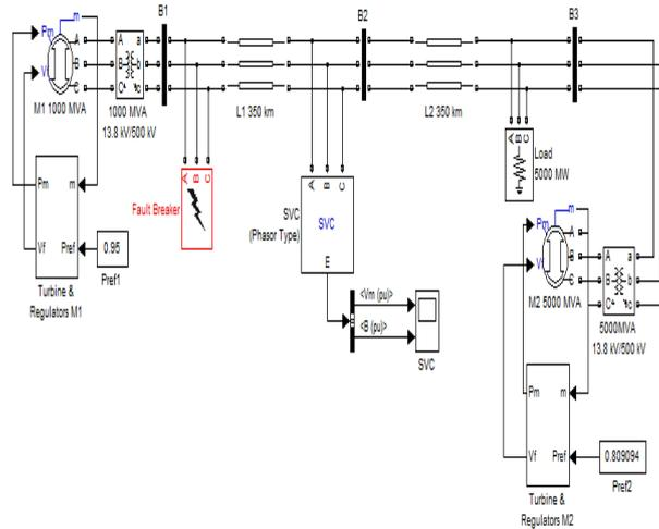
Fig.8. 2-Machine 3-Bus Test system modeled in Simulink/MATLAB
