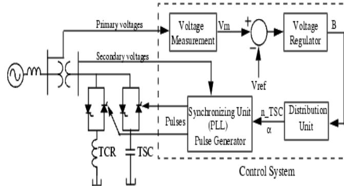
Fig.5. Basic configuration of SVC Control Scheme
