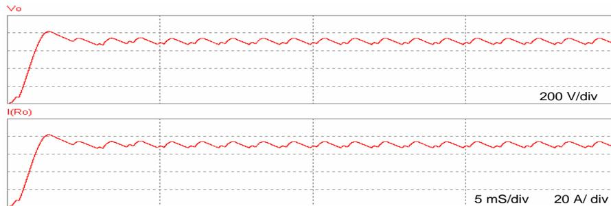
Fig. 9. Output voltage, current waveforms with feedback control.
