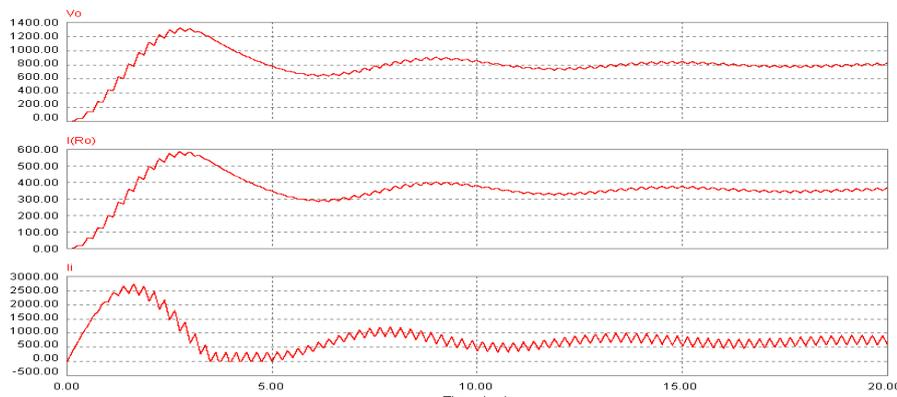
Fig. 7. Input and output waveforms with open loop conditions for synchronous clocking pulse pattern.
