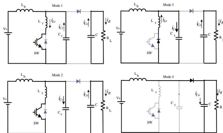
Fig. 5. Boost quasi-resonant operation modes equivalent circuits.
