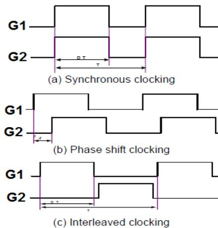
Fig. 2. Gate pulse sequence pattern.
