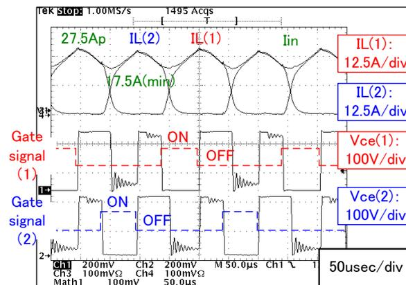
Fig. 13. Inductor currents and gating signals with interleaved clocking.
