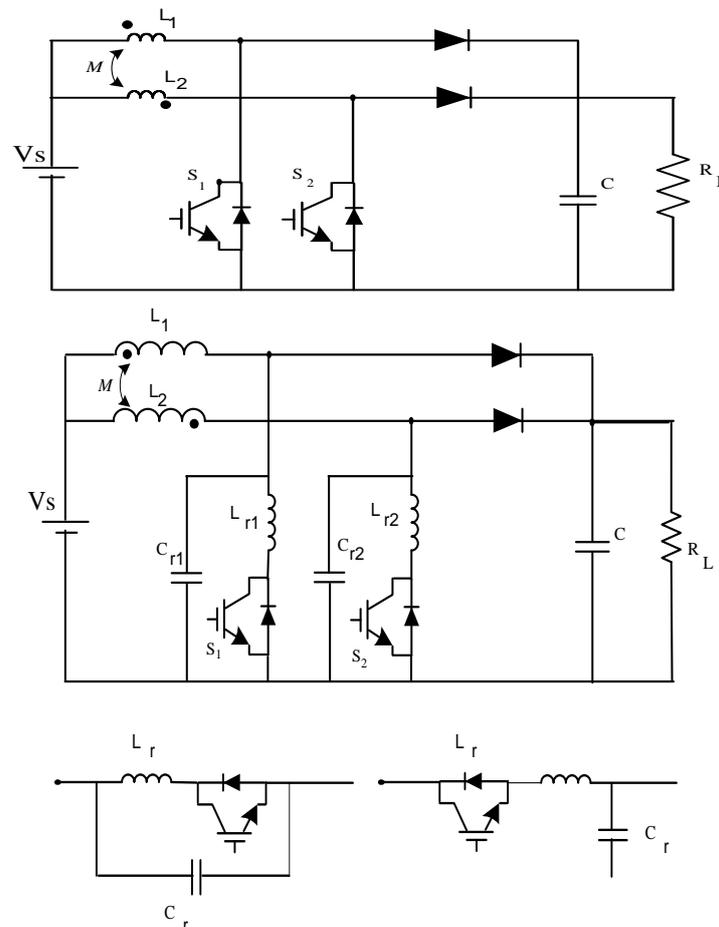
Fig. 1. (a) Hard-switching interleaved Boost DC-DC converter. (b) Soft-switching interleaved Boost DC-DC converter using ZCS PFM cell. (c) ZCS resonant switch cell.
