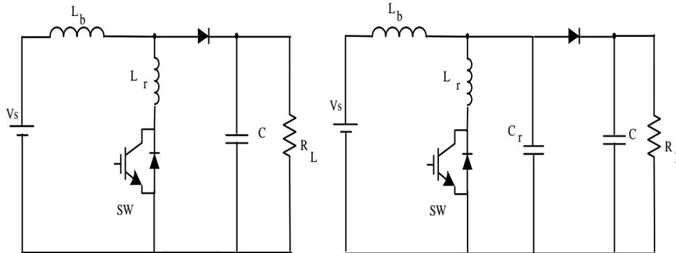
Fig. 3. One unit of ZCS DC-DC converter.
