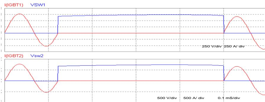
Fig. 8. IGBT current and voltage waveforms and gating signal.
