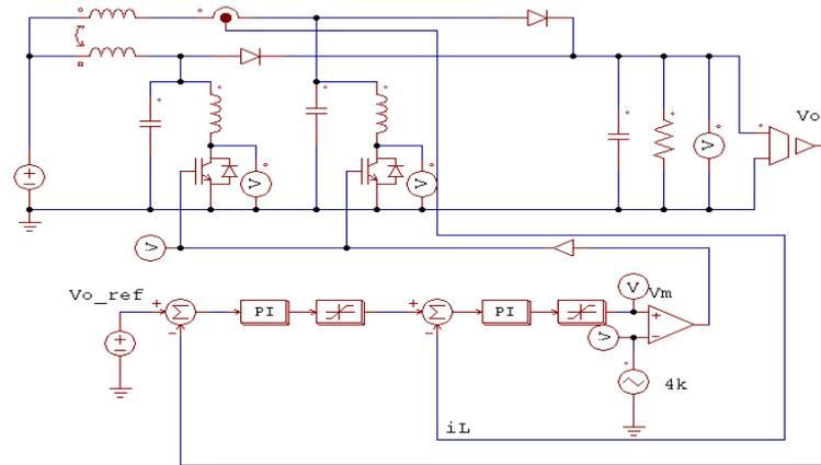
Fig. 6. PSIM model with feedback control.
