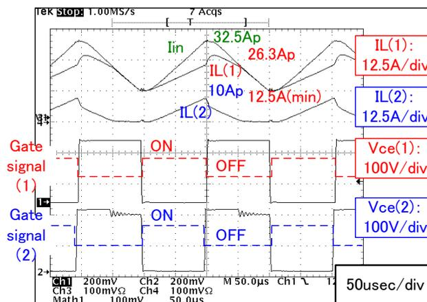
Fig. 14. Inductor currents and gating signals with synchronous clocking.
