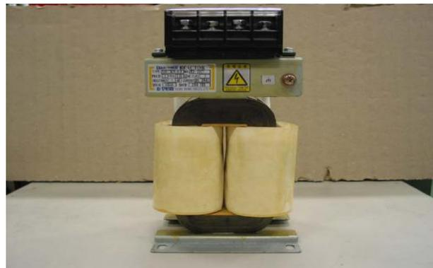
Fig. 12. Two phase coupled inductors.
