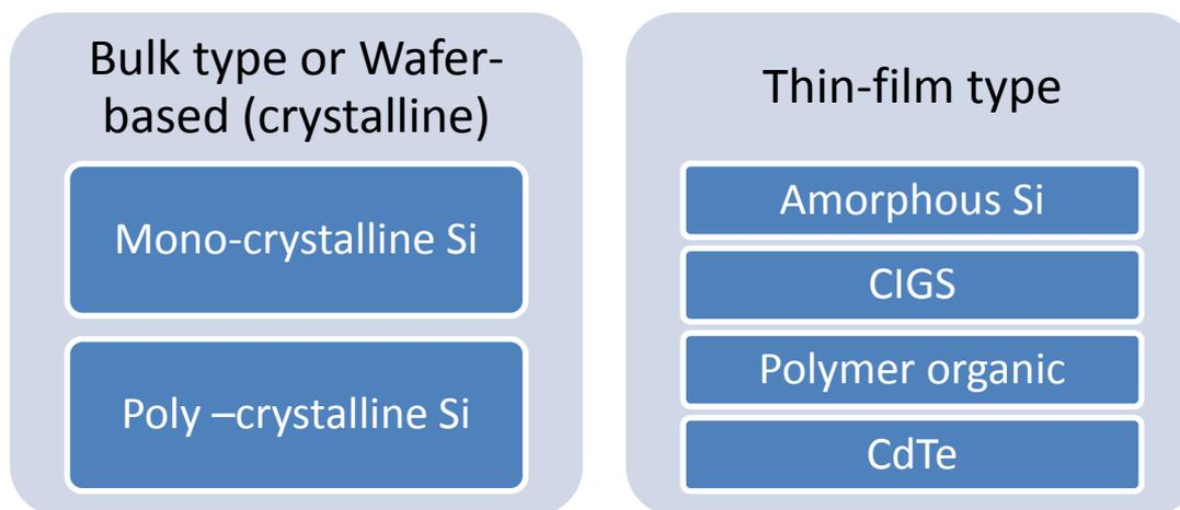
Fig. 2 classification of solar panels
