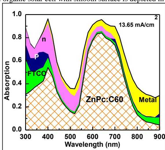
Fig. 5: Quantum efficiency and parasitic absorption plot for optimized substrate (n-i-p) organic solar cell with smooth surface.
