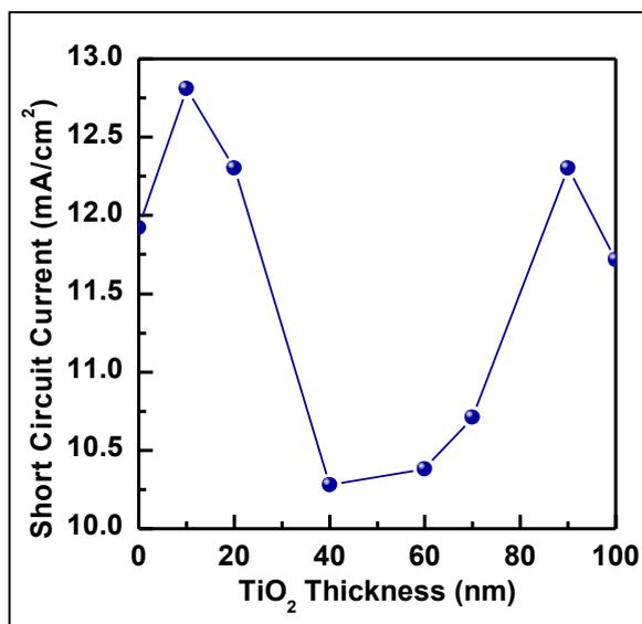
Fig. 4: Short circuit current as a function of TiO<sub>2</sub> thickness for the cell.
