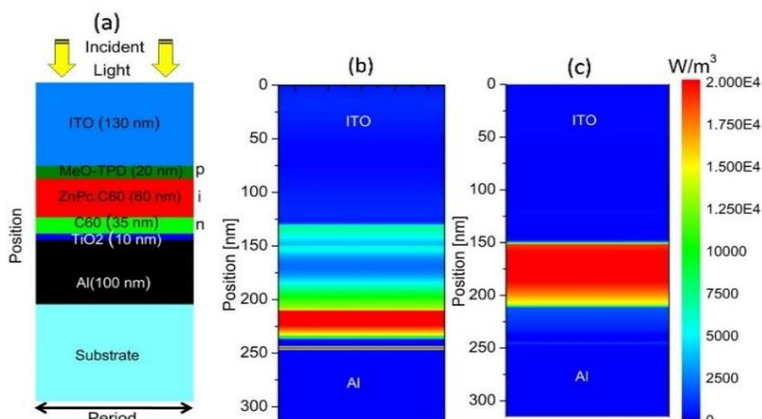
**Fig. 1: (a) Schematic cross section of simulated organic solar cell on smooth substrate; corresponding power loss profile for monochromatic illumination of wavelength (b) 400 nm, and (c) 640 nm.**
