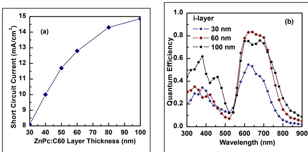
Fig. 2: a) Short circuit current as a function of ZnPc:C60 thickness for the cell. b) Comparison of quantum efficiency for n-i-p organic solar cell with the variation of ZnPc:C60 layer thickness.
