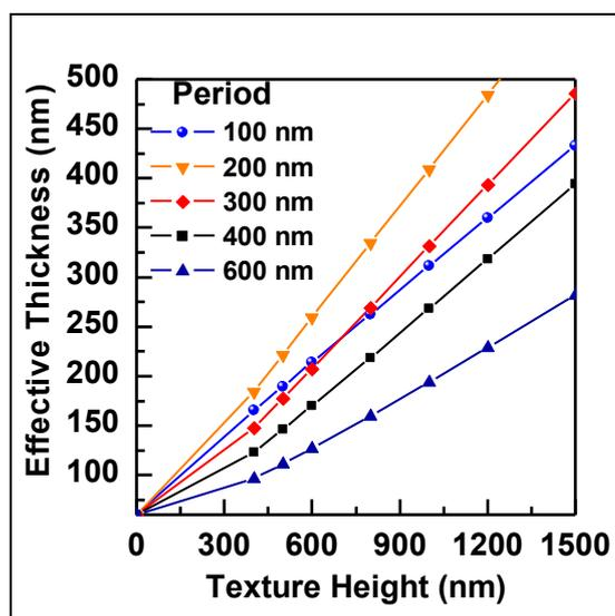
Fig. 7: A comparison of the effective thickness plot of the organic pyramid solar cell with different pyramid period and height.
