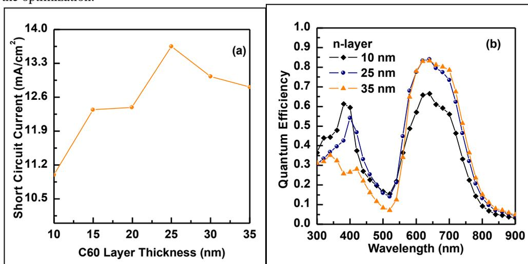
Fig. 3: a) Short circuit current as a function of C60 thickness for the cell. b) Comparison of quantum efficiency for n-i-p organic solar cell with the variation of C60 layer thickness.
