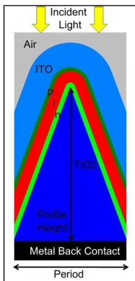
Fig. 6: Schematic sketch of the unit cell of a periodically textured thin-film substrate (n-i-p) organic solar cell for pyramid surface texture.
